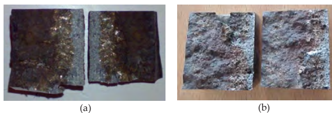
Figure 8. Two photographs showing (a) G material as fractured prior to cleaning and (b) D material after chemical cleaning [7].
